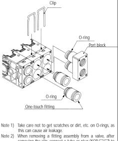
Note 2) When removing a fitting assembly from a valve, after removing the clip, connect a tube or plug (KOP-\_\_\_\_) to the one-touch fitting and pull it out by holding the tube (or plug). If the fitting assembly is pulled out by holding its release bushing (resin part), the release bushing may
